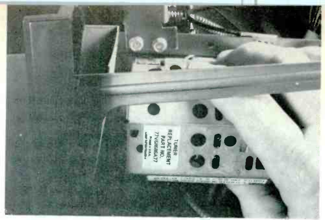
Figure 5. If minor repairs or contact cleaning of the VHF tuner ever becomes necessary, the shield cover slips off easily.
